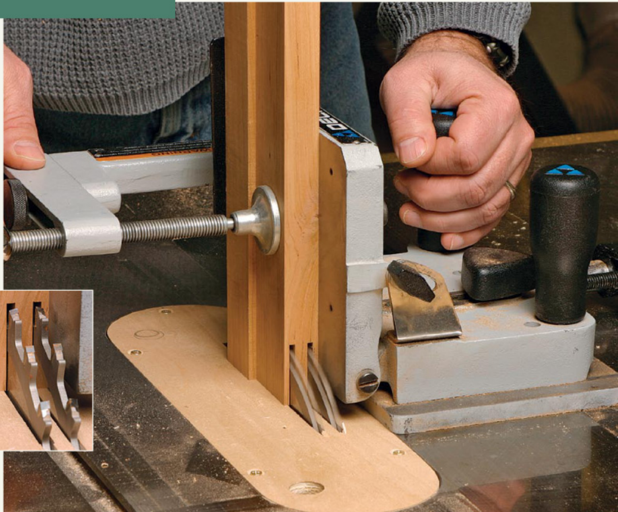
Multiple passes will be necessary for lap joints that span fairly large areas. Use a miter gauge with a stop block clamped to the fence to index the cut.
