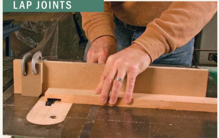
Multiple passes will be necessary for lap joints that span fairly large areas. Use a miter gauge with a stop block clamped to the fence to index the cut.
